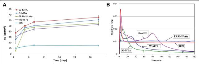
Fig 1 a Microhardness values [kg/mm²] of MTA, ERRM Putty, iRoot FS and IRM at 1, 4, 7 and 28 days after mixing. b Graphical representation of the heat flux generated with time for the different materials
