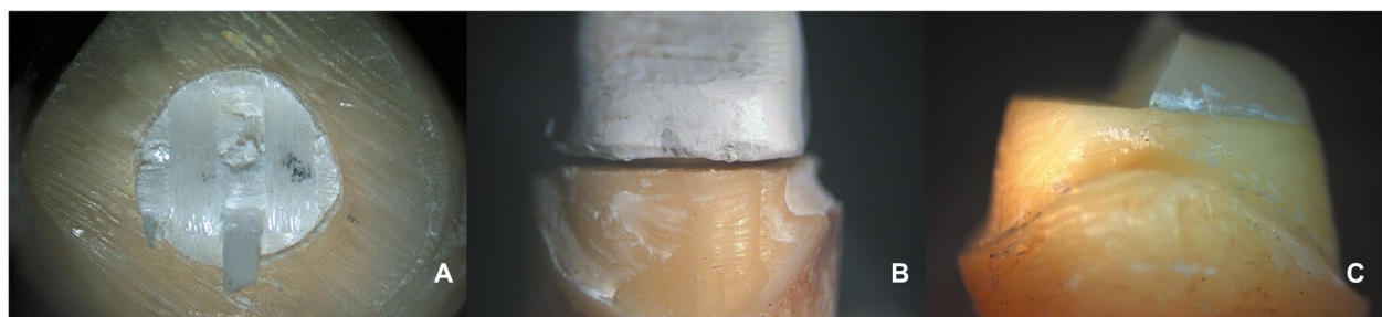
Fig. 6 Stereomicroscope images with 4 X magnification showing favorable fracture patterns in three tested groups. A FRC sample displayed core separation. B PEEK sample exhibited post and core dislodgment. C PICN sample fractures confined within the core
