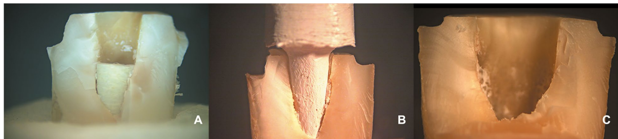
Fig. 7 Stereomicroscope images with 4 X magnification showing unfavorable fracture patterns in three tested groups: A , FRC sample displayed fractures in both post and core restoration and vertical root fracture below CEJ. B , PEEK sample exhibited vertical root fracture below CEJ, while post and core restoration remained intact. C , PICN sample showed fractures in both post and core restoration, and vertical root fracture below CEJ
