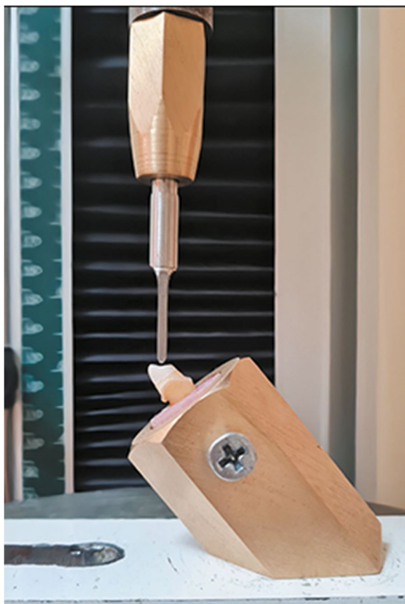
Fig. 2 Compressive static load applied 45° palatal to specimen
