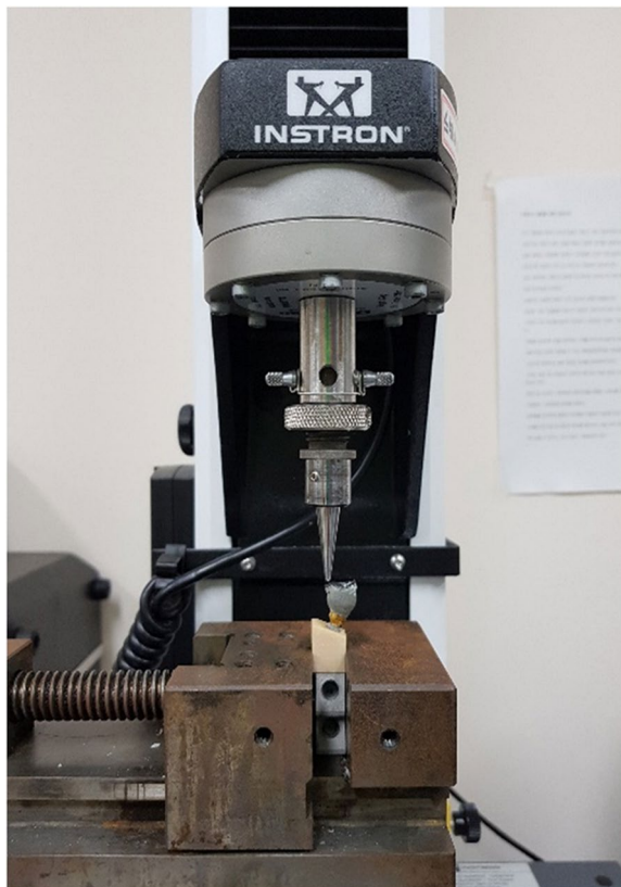
Fig. 8 Universal testing machine used in this study (Instron 3345, Instron Co., Norwood, Massachusetts)
