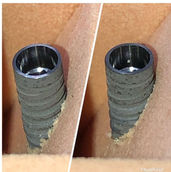
Fig. 2 Implants placed without lateral contacts (“step” osteotomies) in dense artificial bone, representing implant placement in a fresh extraction socket with only apical stability. GM™ Drive™ implants placed at 5 mm and 7 mm, respectively
