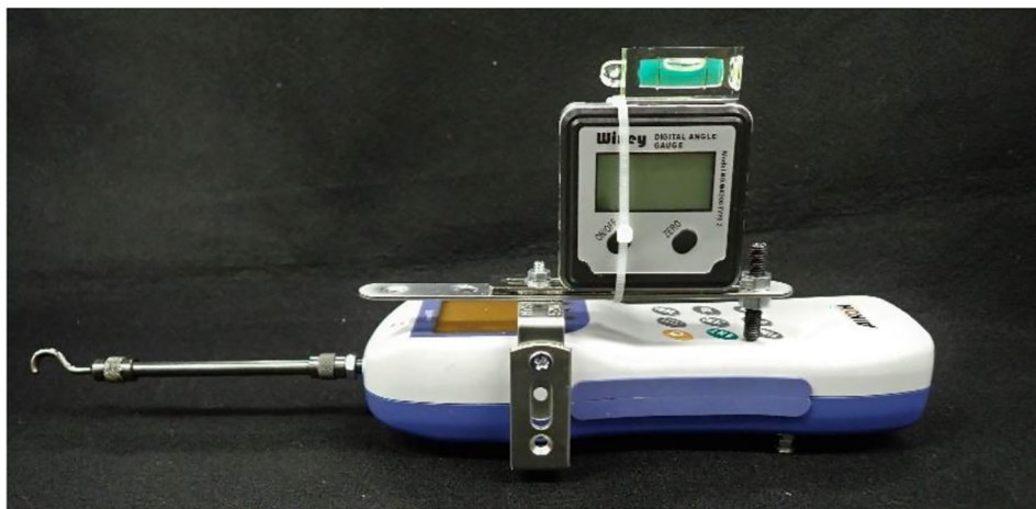
Fig. 2 The measuring device with angle meter attached
