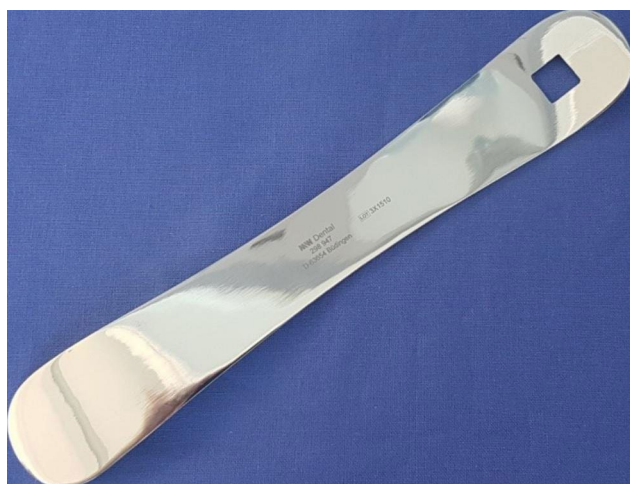
Fig. 1 Sterilizable stainless steel template for standardized sampling within an area of 1 cm 2
