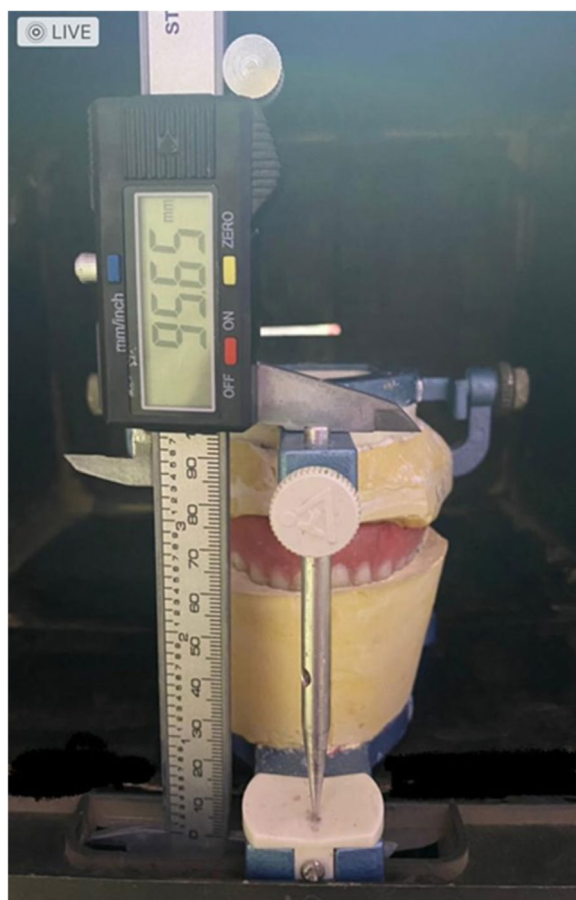
Fig. 2 shows the digital calliper was used to measure the distance between upper and lower member of the articulator at the constant predetermined position (final measurement)
