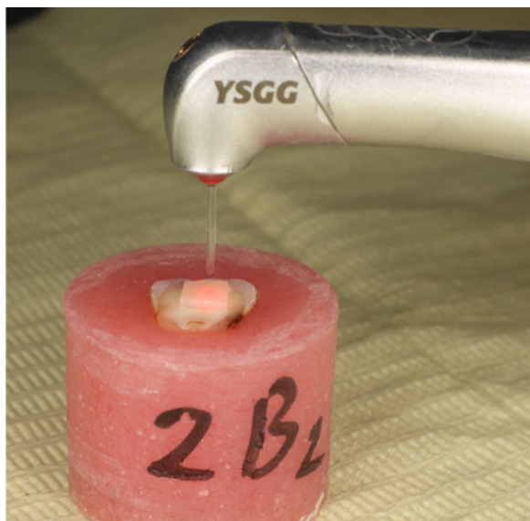
Fig. 2 LASER application perpendicular to ceramic surface
