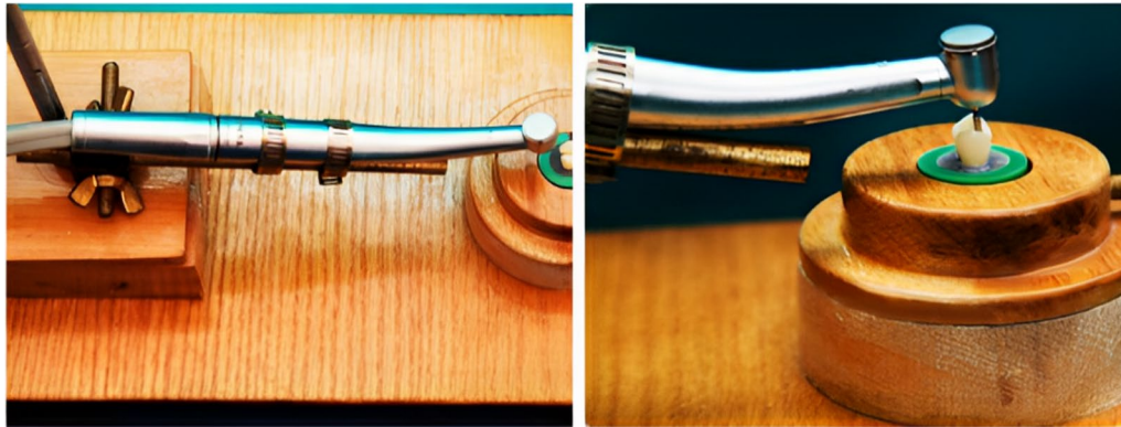
Fig. 3 A specially designed apparatus to which the high-speed handpiece was affixed to standardize the cavity preparation
