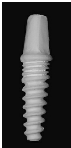
Fig. 3 Customized one-piece zirconia implant before sintering
