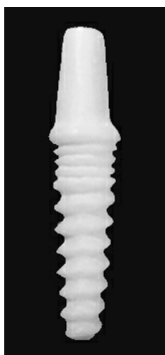
Fig. 4 Customized one-piece zirconia implant after sintering
