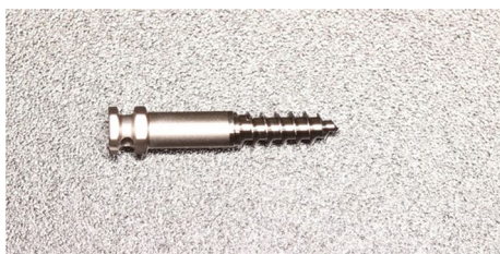
Fig. 1 Mini-implant (Cibei, Ningbo, China, 2 mm in diameter and 13 mm in length)
