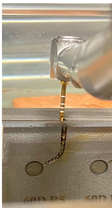
Fig. 1 A custom-made stainless-steel canal with dimensions that are larger than the dimensions of F2 instrument by 0.1 mm in width. The canal has 60° curvature angle, 5 mm curvature radius and curvature center located 5 mm coronal to the instrument tip
