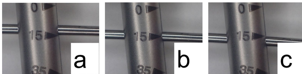
Fig. 3 Location of the beam on the scale. a leading edge, b center, c trailing edge
